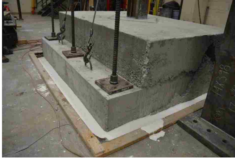
Figure 3-26: Specimen Immediately after Being Placed in HYDROCAL
