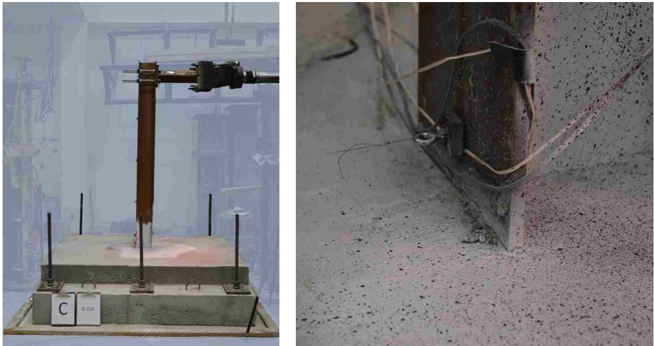
Figure 4-5: Specimen A1 at 0.01 Drift
