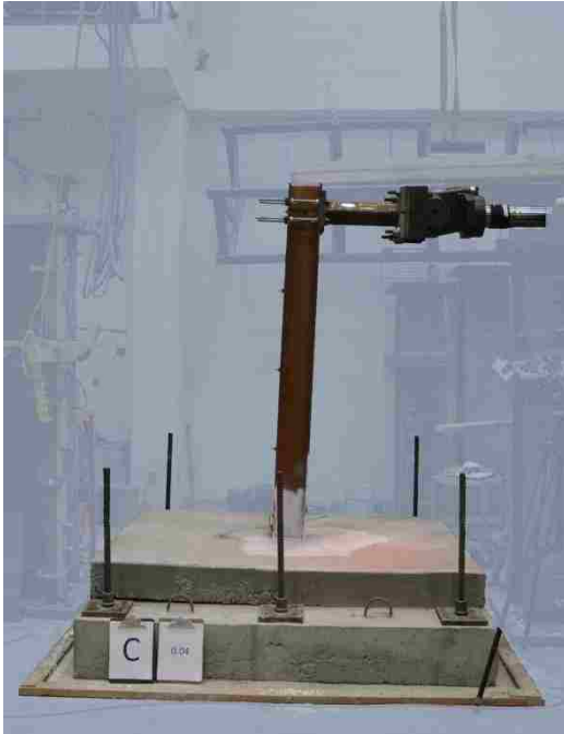
Figure 4-8: Specimen A1 at 0.04 Drift
