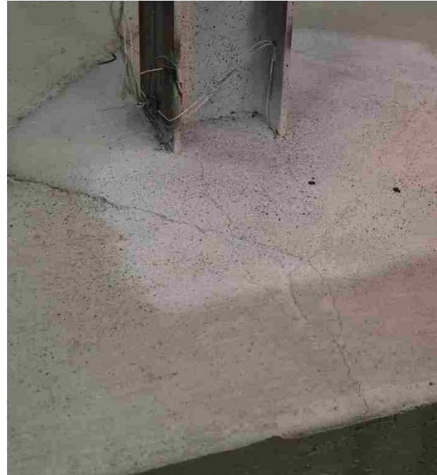
Figure 4-8: Specimen A1 at 0.04 Drift
