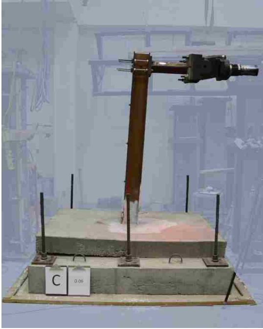
Figure 4-10: Specimen A1 at 0.06 Drift
