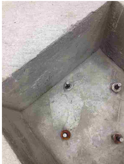
Figure 3-22: Shifted Block-out on Specimen E
