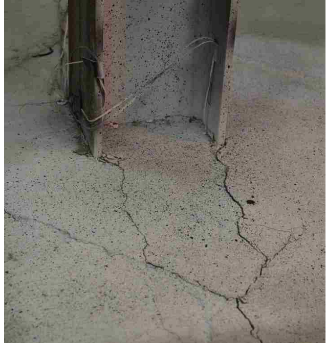
Figure 4-10: Specimen A1 at 0.06 Drift
